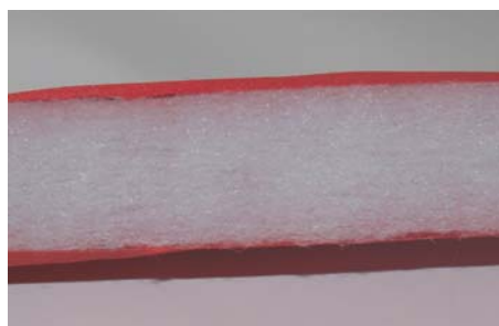
Cut of insulated duct
