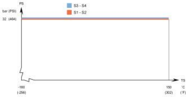
ACH16 - PED approval pressure/temperature graph
